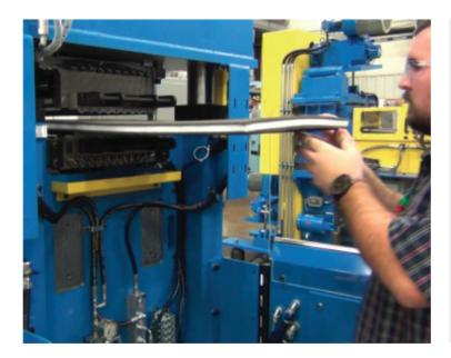
The leveler also features Machine Concepts' patented Roll Cleaning System. When processing surface-critical materials, keeping the work rolls clean is paramount to producing a high-quality product. The leveler has the ability to open a full 6 inches, allowing easy access to the work rolls.
