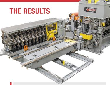
The 72" wide, 5-high configured cassette-style roller leveler utilizes two individual roll cassettes with 1.50" and 2.25" diameter work rolls.
